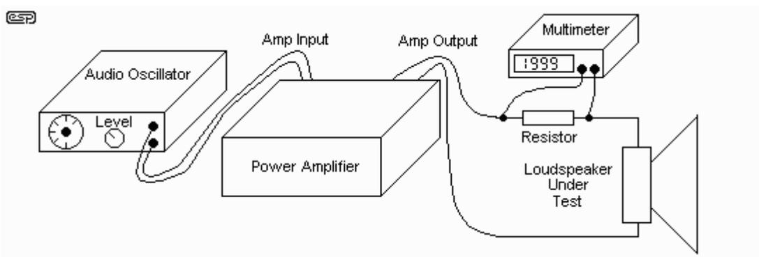
Figure 2 - Measuring the Main Speaker Parameters
