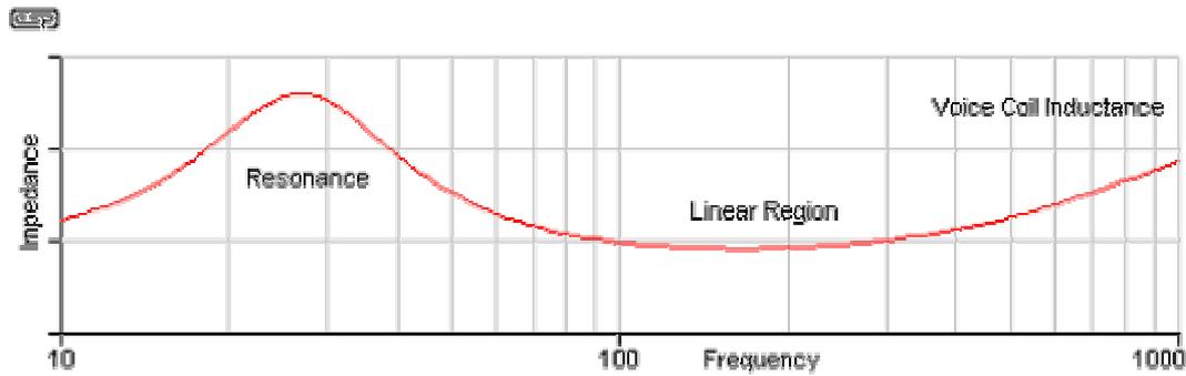
Figure 1 - Loudspeaker Impedance Curve
