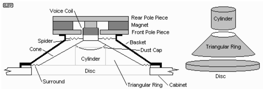
*Figure 4 - Determining the Volume of the Cone*
